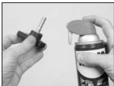
(J) Lubricate the Cutting Head Adjustment Knob.
