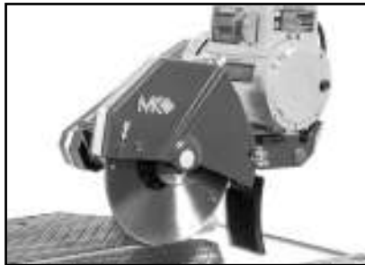
(B) Inspect Diamond Blade for damage.
