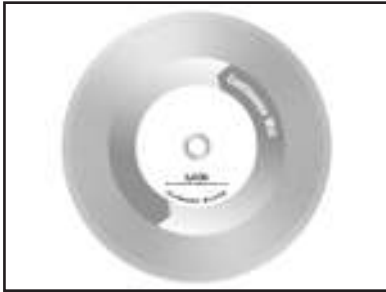
(A) Check for Smoothness or "Glazing" (Dress blade if needed).
