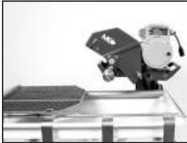
(B) Raise the Blade Guard by loosening the wingnut.
