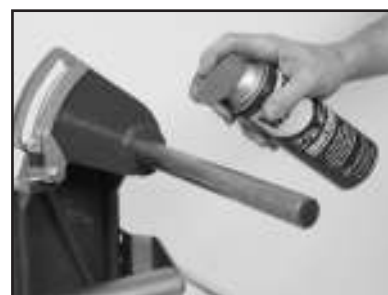
(L) Lubricate the Cutting Head Pivot Shaft.
