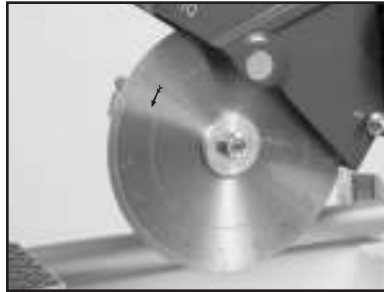
(B) Check for proper blade rotation.
