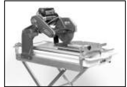
(C) Pull Movable Cutting Table to front of Tile Saw.
