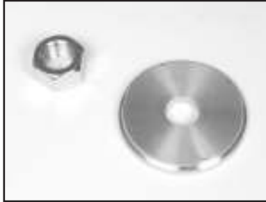
(B) Lubricate the Outer Flange and Retaining-nut.
