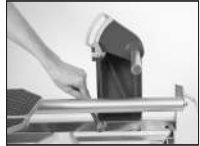
(C) Loosen the Post Support and retaining bolts.
