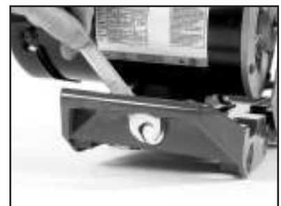
(I) Loosen the Motor Adjustment Strap
