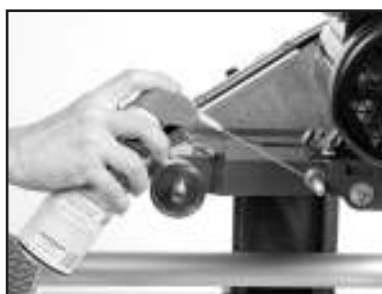
(H) Lubricate the Blade Guard Pivot Shaft.
