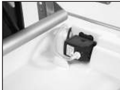
(B) Place Water Pump in Water Pan. Fill the Water Basin until water completely covers the Water Pump suction.
